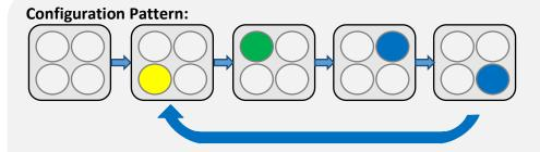
During USB configuration, the LEDs will flash in a clockwise manner. This process will continue for 2-5 minutes during the configuration process. Afterwards, either the success pattern or the error pattern will display on the LEDs.
