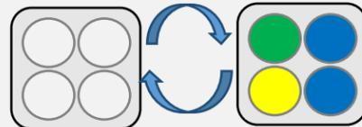
This LED pattern is used to indicate that the configuration has completed successfully. All four LEDs will flash simultaneously once per second. When this pattern shows remove power from the Amphion, remove the USB stick, and re-apply power to restart the newly configured Amphion.
