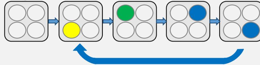
During USB configuration, the LEDs will flash in a clockwise manner. This process will continue for 2-5 minutes during the configuration process. Afterwards, either the success pattern or the error pattern will display on the LEDs.
