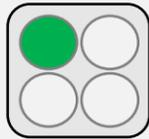
**System LED:** The green LED represents the status of the device. When the A14-N has completed booting it will flash once per second.
