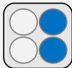
**Tunnel LEDs:** An active blue LED shows that the A14-N (red box) is connected to either an A14-H (green box) or A14-K (orange face). If both blue Tunnel lights are off, it usually indicates that the Amphion does not have connection.
