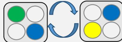
This LED pattern shows that there was a problem during configuration. The LEDs will flash in an "X" pattern to indicate an error. It usually means that there was an error reading the configuration file from the USB stick. Common causes of this include a bad USB stick, a corrupt configuration file, or a USB drive with more than two files with the string "PATCH" in their filenames.
