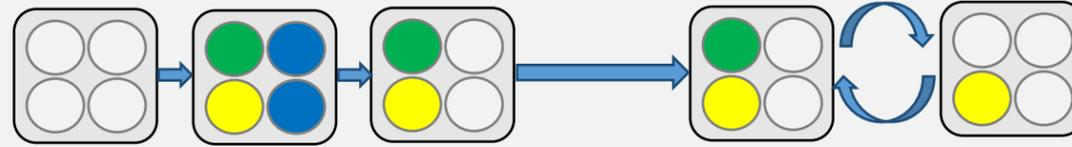
The Amphion can take up to 5 minutes to start. Once booted, the green System LED will begin to flash once per second. The blue LED will begin to flash when the connection to the A14-H (green box) or A14-K (orange face) is established.
