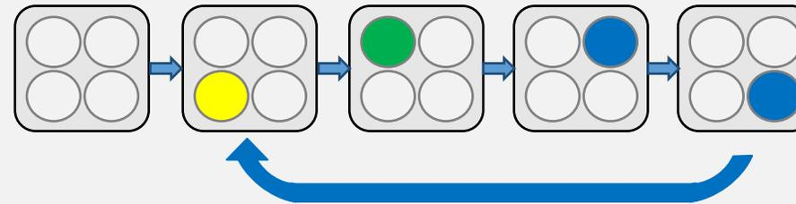
During USB configuration, the LEDs will flash in a clockwise manner. This process will continue for 2-4 minutes during the configuration process. Afterwards, either the success pattern or the error pattern will display on the LEDs.
