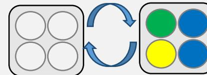
This LED pattern is used to indicate that the configuration has completed successfully. All four LEDs will flash simultaneously once per second. When this pattern shows, remove the USB stick. The newly configured Amphion will automatically restart itself and then it will be ready to use.
