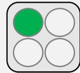
**System LED:** The green LED represents the status of the device. When the Amphion has completed booting it will flash once per second.
