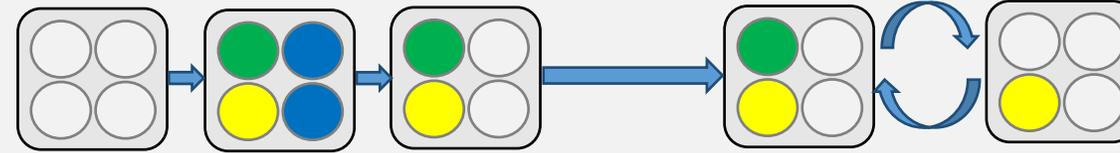
The Amphion can take up to 2 minutes to start. Once booted, the green System LED will begin to flash once per second. A blue LED will begin to flash when the Amphion S14-N establishes a connection to an S14-H, A14-H, or A14-K.
