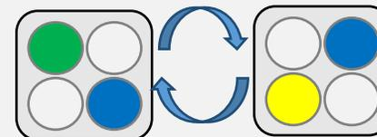
This LED pattern shows that there was a problem during configuration. The LEDs will flash in an "X" pattern to indicate an error. It usually means that there was an error reading the configuration file from the USB stick. Common causes of this include a bad USB stick, a corrupt configuration file, or a USB drive with more than two files with the string "ei3" in their filenames.
